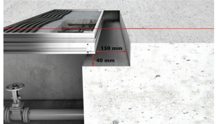
**Step 2:** A minimum rebate of 150mm wider than the over frame size and 40mm deeper than the over frame height of the access cover is to be provided for bedding and haunch material.
