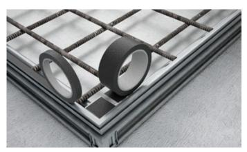
**Step 3:** Ensure upper surfaces of the cover and frame, weldable PVC trim, joints and locking areas are protected from accidental spillages or ingress of installation materials. This will help reduce the need for cleaning prior to vinyl floor welding or at the end of the installation.
