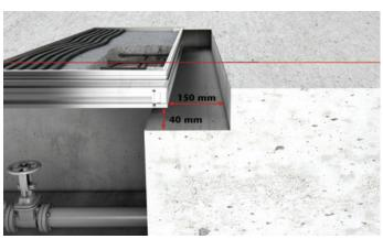
**Step 2:** A minimum rebate of 150mm wider than the over frame size and 40mm deeper than the over frame height of the access cover is to be provided for bedding and haunch material.
