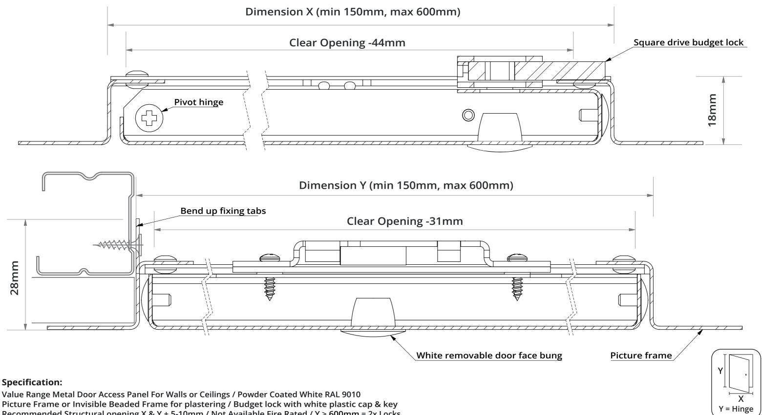
Picture Frame or Invisible Beaded Frame for plastering / Budget lock with white plastic cap & key Recommended Structural opening X & Y + 5-10mm / Not Available Fire Rated / Y > 600mm = 2x Locks
